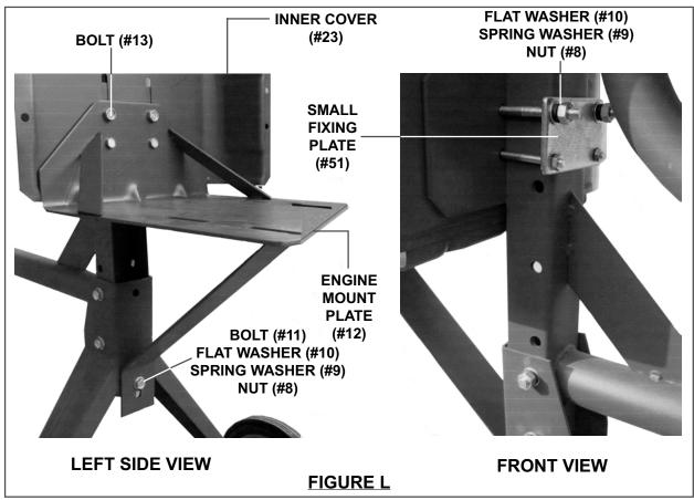
15. Align the mounting hole in the Angle Brace of the Engine Mount Plate (part #12) with the mounting hole in the Hinge Bracket (part #2). Then, secure the Angle Brace to the Hinge Bracket with one Bolt (part #11), one Flat Washer (part #10), one Spring Washer (part #9), and one Nut (part #8).
